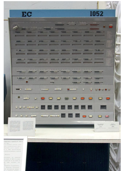
The control unit of an ES-1052.
